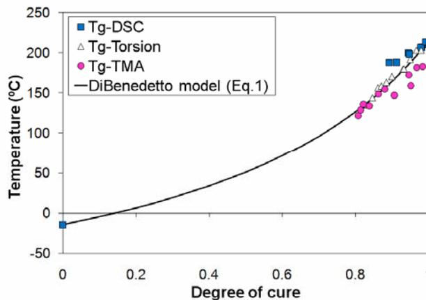
Fig. 1 Comparison of glass transition temperature measured with different methods.
