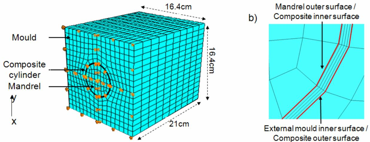
Fig. 4 a) Finite element geometry of the composite cylinder in the mould and symmetric boundary conditions – b) Details of the composite cylinder through thickness mesh.
