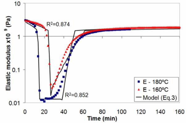
Fig. 3 Comparison of the experimental and predicted elastic modulus data in time.
