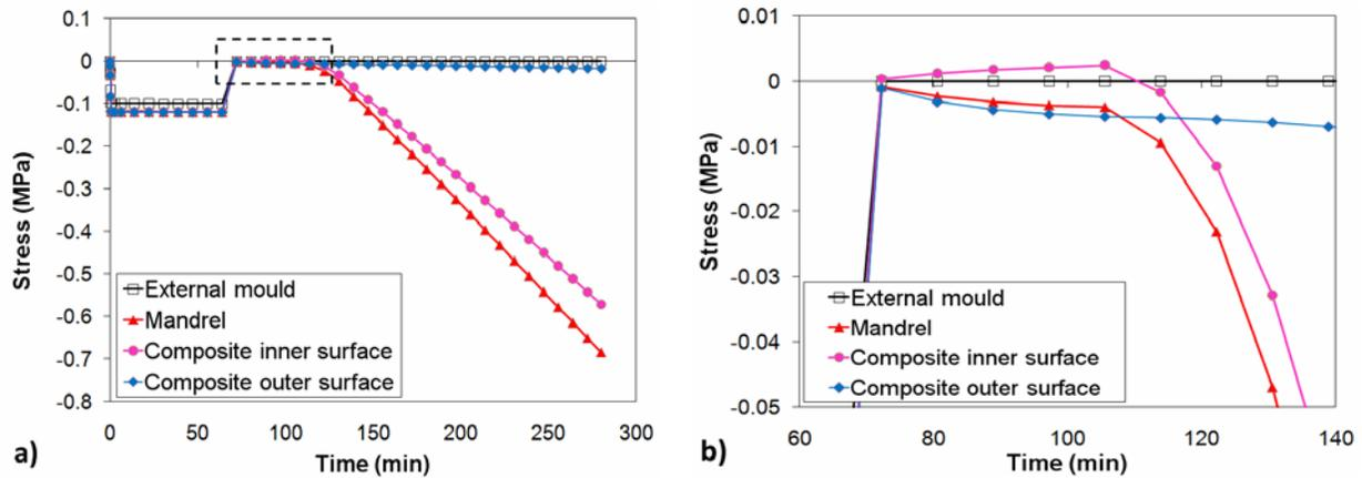
Fig. 7 Stress evolution at the interfaces: a) during the whole cure cycle; b) at the end of the isotherm.
