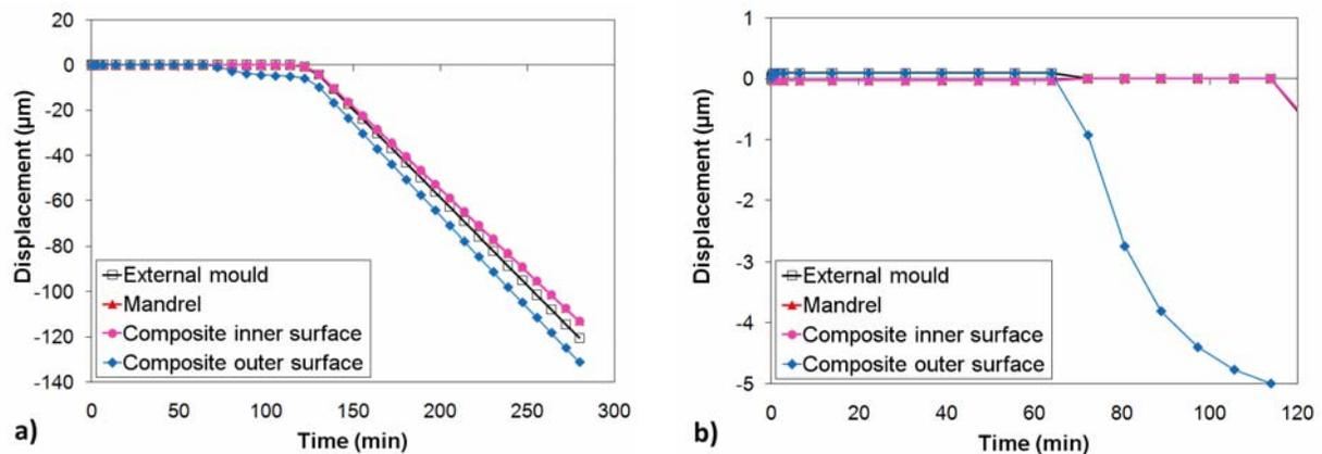
Fig. 8 Displacement evolution at the interfaces: a) during the whole cure cycle; b) during the isotherm.
