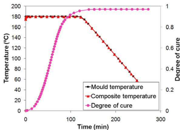
Fig. 5 Temperature and degree of cure evolution at the center of the composite.
