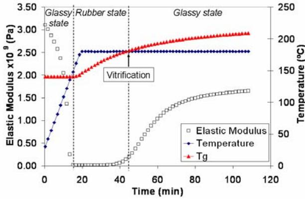
Fig. 2 Evolution of the elastic modulus with temperature and time.
