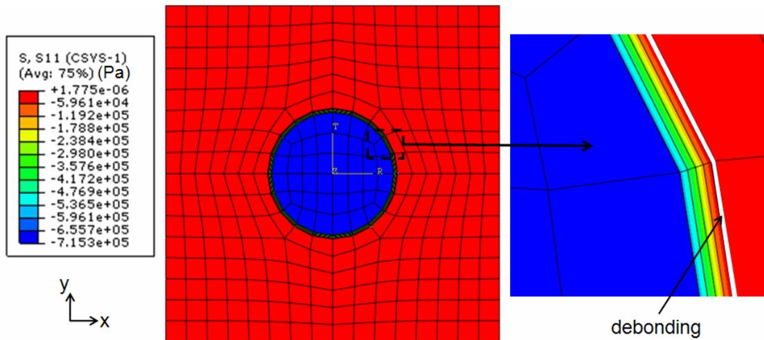
Fig. 9 Stress distribution in the radial direction at the end of the cure cycle at 25°C (scale factor x20).
